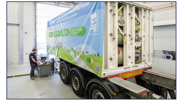
Hydrogen tube trailer – ready for operation test
